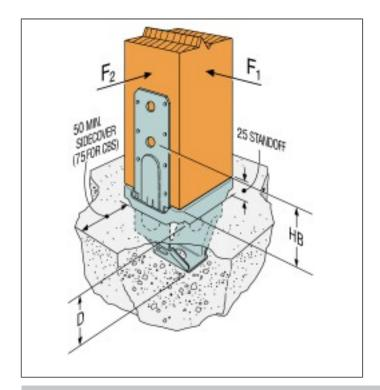
The PBS post base is installed into wet concrete and features a 25mm standoff to help prevent moisture induced decay to the timber post.
