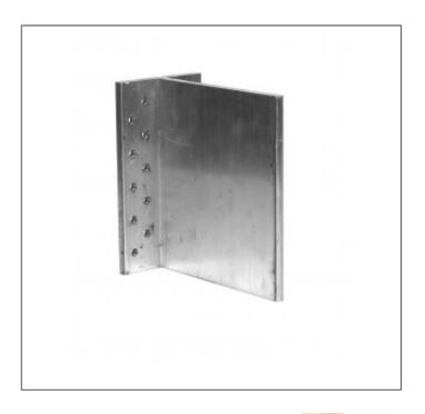
The BTALU concealed hanger is one solution to connecting timber members together without seeing the connector. It is designed to be fixed to the header timber and then fully inserted into a slot in the in-coming beam, and held in place with dowels. Holes are drilled through the timber and fin of the BTALU, allowing accurate alignment. his method provides an aesthectically pleasing connection for feature beams.
