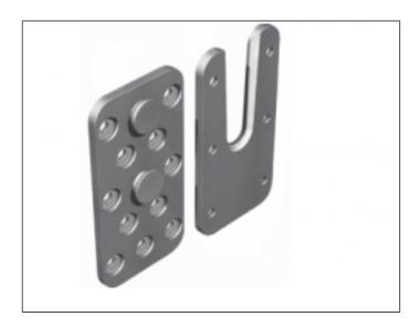
The first part of the connector is fixed into a pocket on the header timber with nails and the second part on the end of the incoming beam with screws. No slots or dowel holes are necessary, speeding up production.
